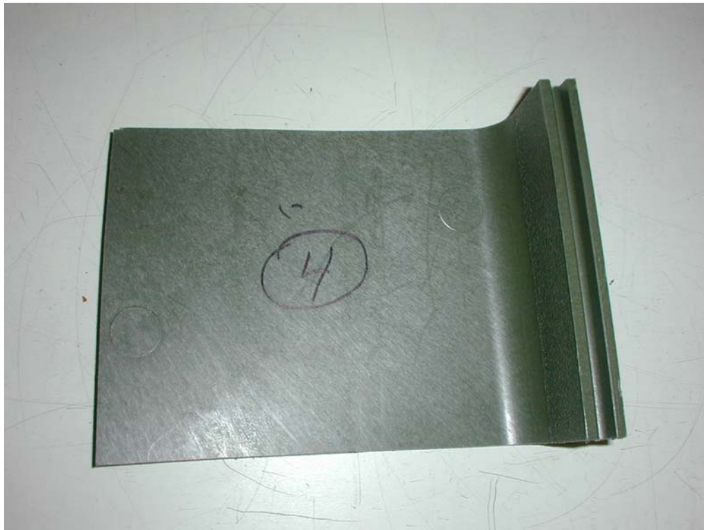
Photograph 4-5: Green Plastic Sample upon completion of the incubation period
